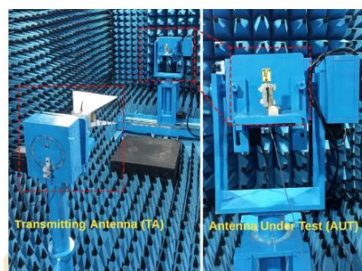
Figure 3.12. Experimental Setup for Radiation Pattern Measurement.
